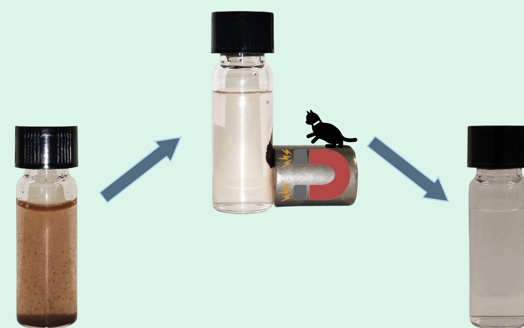
Fig 3. Picture of Magnetic MOF in water, before (left) and after (center) the application of a magnetic field and the removal of the magnetic powder (right)
